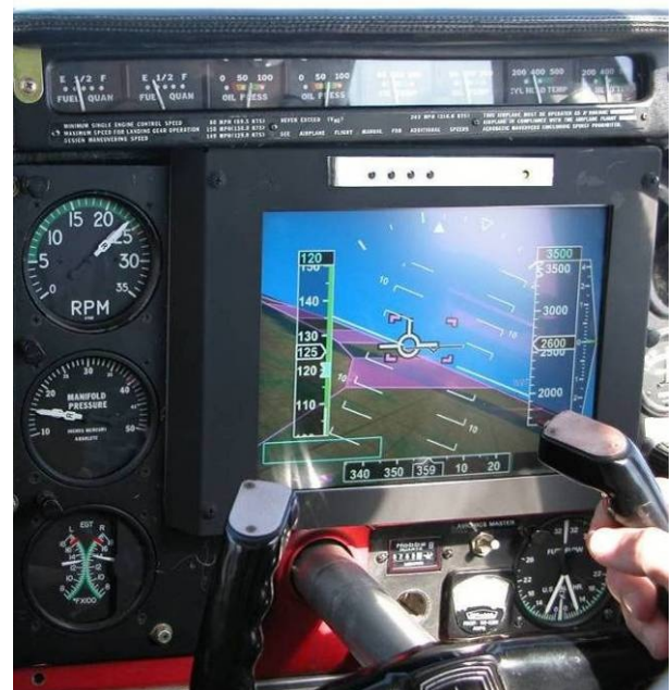
Figure 2. PFD Installation in Piper Aztec.
